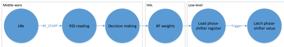
Figure 14 Beamformer state machine
