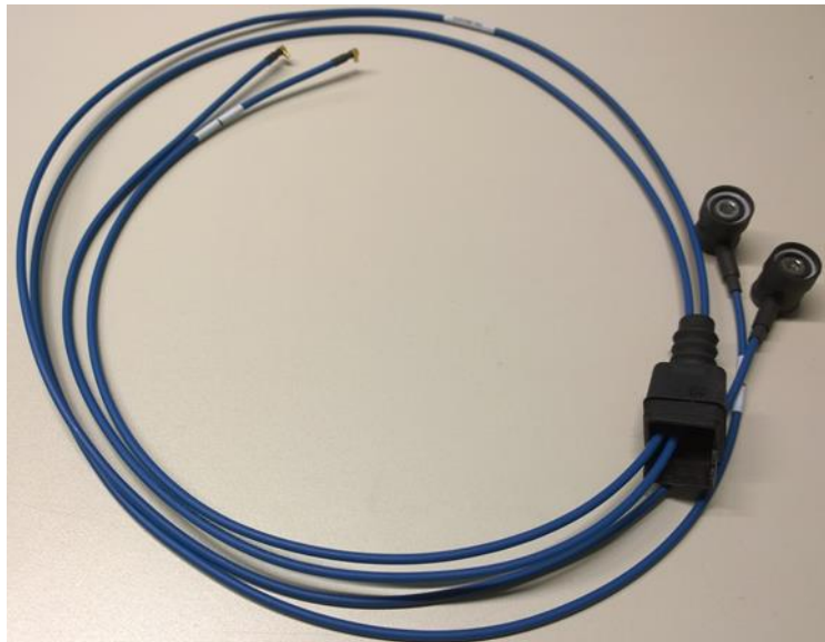
Figure 15. Sub 6 GHz IF cable that connects the TRX unit to two RF boards
