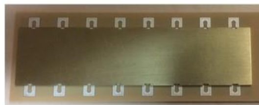
Figure 5: Manufactured antenna array with 16 RF ports
