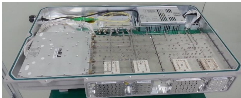
Figure 24: RF and Antenna Unit (RU)
