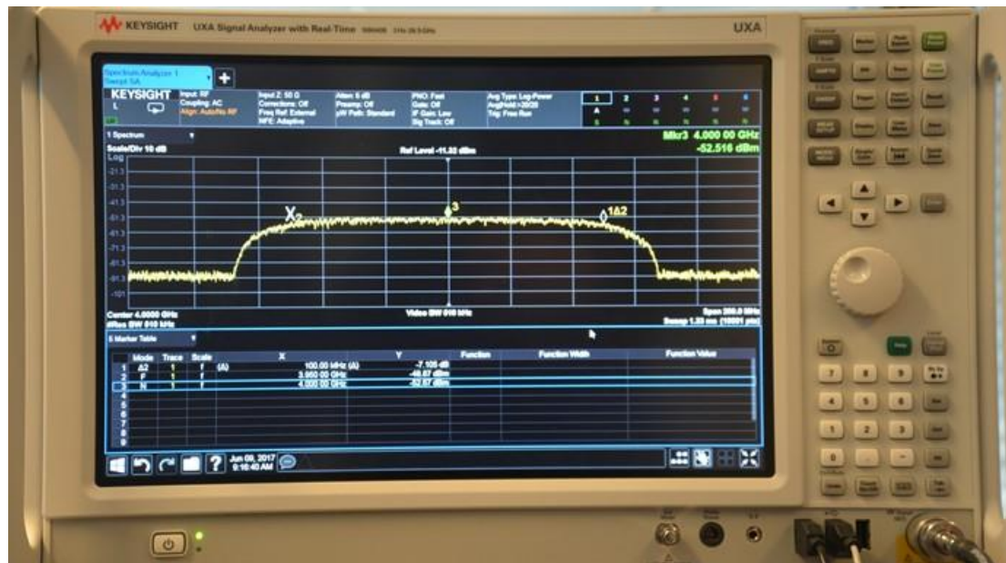
Figure 8: Example of test signal: 100MHz single channel 16QAM modulated signal
