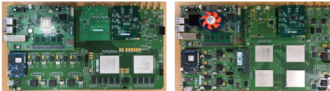
Figure 21 NodeB (DU) Baseband platform and TE Baseband platform
