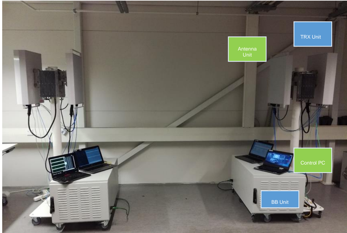
Figure 3 5GCHAMPION EU mmW Backhaul testbed
