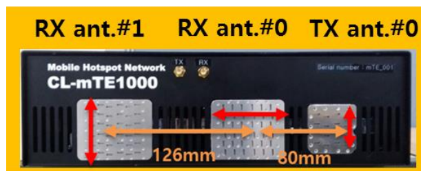
Figure 31 mTE antenna configuration
