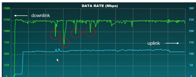
Fig. 9. Measured data throughput during 2.4 km run
